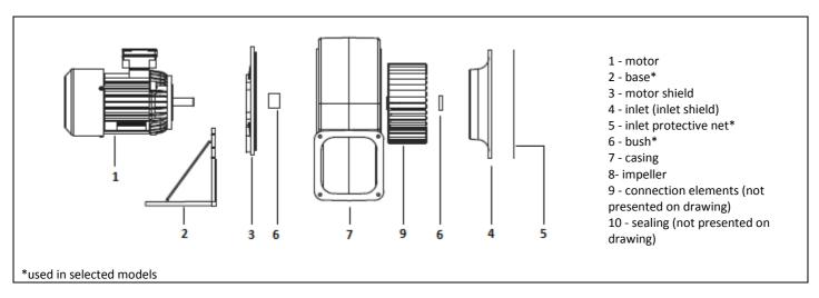
Fan casing, base, inlet shield (2, 3, 4) are made of painted cast aluminum. Inlet (4) is made from painted cast aluminum / galvanized steal. Inlet protective net (5) is made from galvanized steal. Bushing (7) is made from steal, stainless steal. Impeller (8) is made from galvanized steal and connection elements (galvanized steal, stainless steal). Connection elements are made from galvanzied steal. For sealing - sealing paste has been used.
