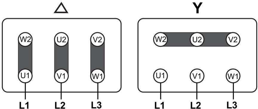
Fig. 35: Terminal assignment for delta and star connection
