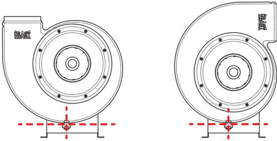
Fig. 30: Proper position of the casing drain
