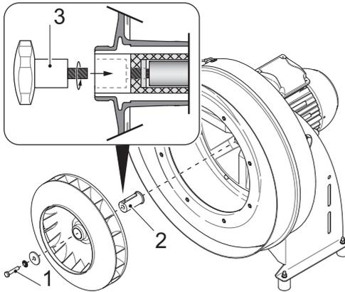
Fig. 39: Removing impeller
