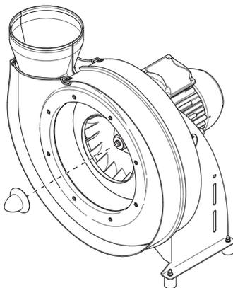
Fig. 38: Removing hub cap
