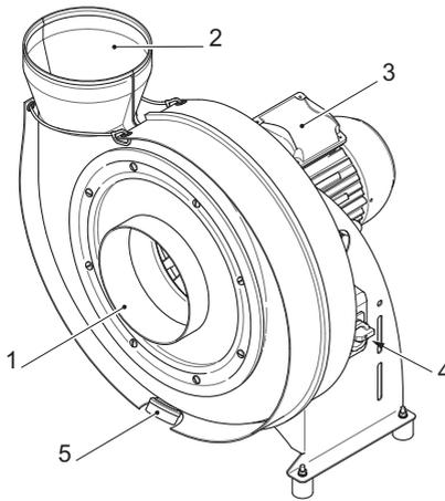
1. Inlet connection (suction side): Connection to supply air ductwork with sleeve.
