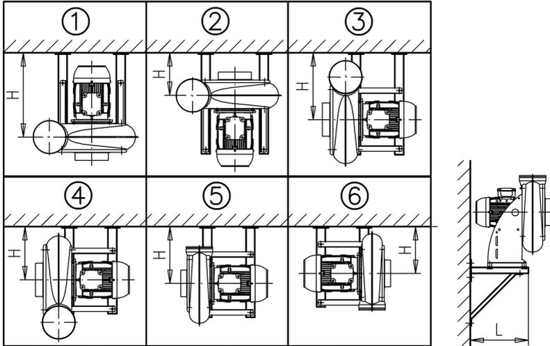
Fig. 27: Mounting position on the wall bracket
