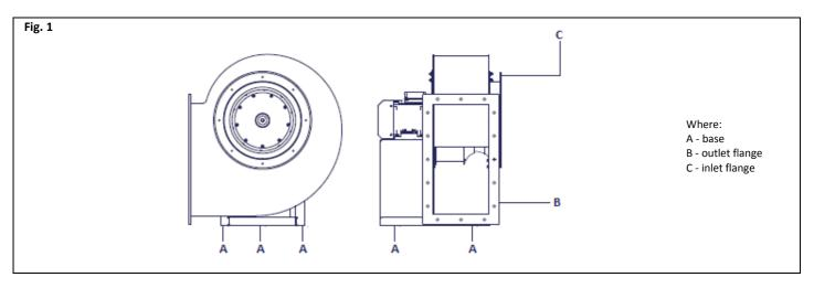
•Supporting construction has to be solid enough in order to carry the weight of the fan and generated vibration (including fan damage). The fan cannot be exposed to vibration.
