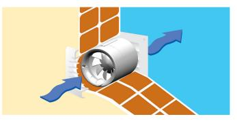
Installation inside the wall to exchange heat between adjoining rooms and exhaust air from the spaces.
